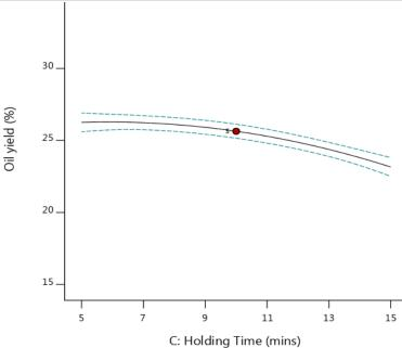
Fig. 8: Effect of holding time (mins) end point temperature (<sup>0</sup>C) on oil yield with the Electric Field strength of 12 (V/cm) and end point temperature of 50 <sup>0</sup>C
