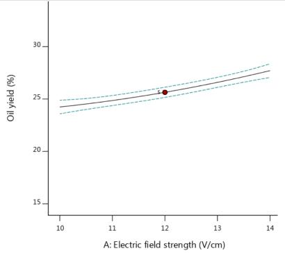
Fig. 6: Effect of Electric Field strength (V/cm) on oil yield with the end point temperature of 50<sup>o</sup>C and holding at 10 mins
