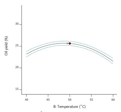
Fig. 7: Effect of end point temperature (<sup>0</sup>C) on oil yield with the Electric Field strength of 12 (V/cm) and holding at 10 mins.
