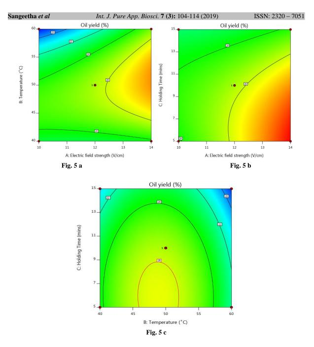
Fig. 10: Two-dimensional response surface contour plots showing the experimental factors and their mutual interactions on oil extraction: (a) Y = f (A, B, 10); (b) Y = f (A, 50, C); (c) Y = f (12, B, C)
